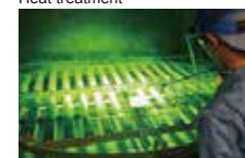
NDT (penetrant inspection)
